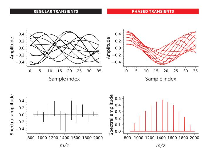
**Transients vs. aFT:** Fourier transform (FT) of a regular FTMS transient whose components have diverse phases (left, top) yields a mixed-mode mass spectrum (left, bottom) that requires post-processing for it to be represented in absorption mode (aFT). Right panels: FT of transients with in-phase ion signals (right, top) generates mass spectra directly in absorption mode (right, bottom).
