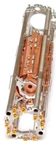
2X NADEL ICR cell design is based on the open-ended cylindrical cell (Ultra™ ICR cell from Thermo Scientific). The patented 2X NADEL ICR cell consists of four wide aperture excitation grid-electrodes and four narrow aperture detection electrodes, thus NADEL ICR cell [1].
